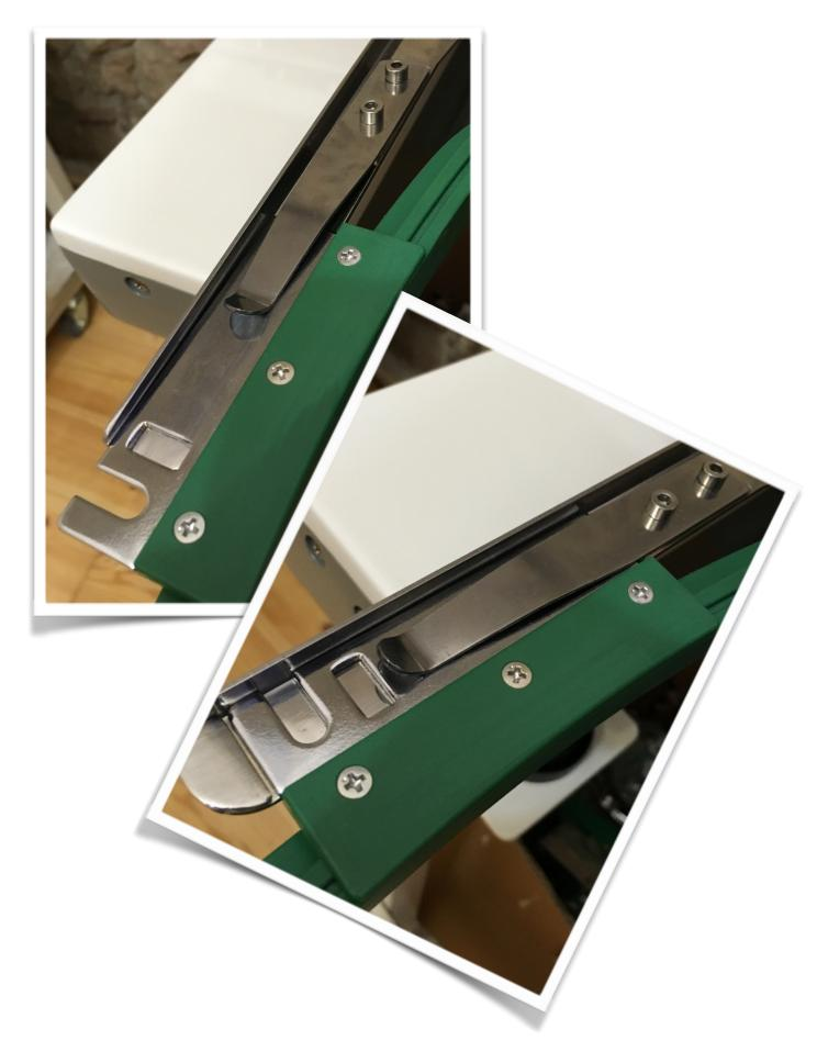
New metal plates on top of the metal stand -The machine can be easily transported -The setting up and dismantling of the machine is much faster -
